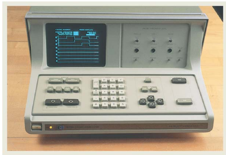
Figure 10 Timing analysis of an AND gate: (a) waveform sketch; (b) actual logic analyzer display.
