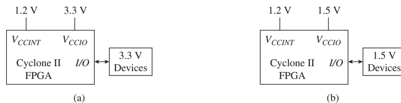
Figure 35 Interfacing an FPGA to different I/O devices: (a) the 3.3 V V_{CCIO} I/O configuration; (b) the 1.5 V V_{CCIO} I/O configuration.
