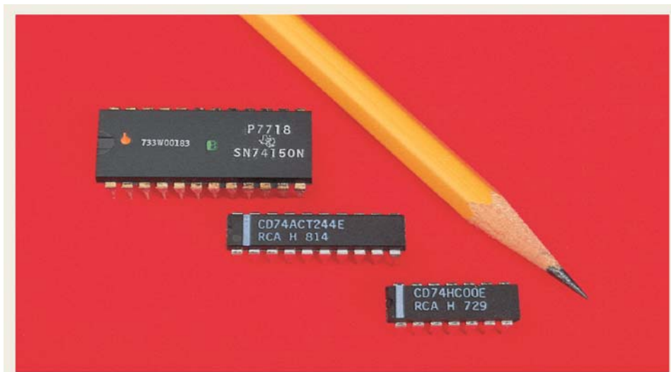
Figure 40 Photograph of three commonly used ICs: the 74HC00, 74ACT244, and 74150.
