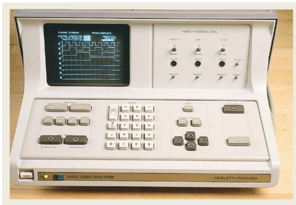
Figure 12 MOD-16 ripple counter: (a) Block diagram; (b) waveforms; (c) counter displayed on a logic analyzer.
