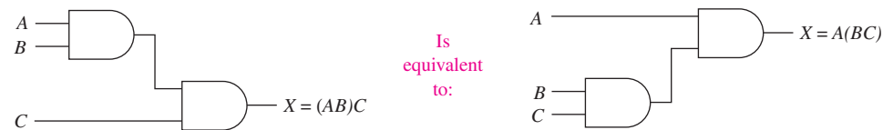
Figure 11 Using the associative law of multiplication to rearrange the grouping of AND gates.
