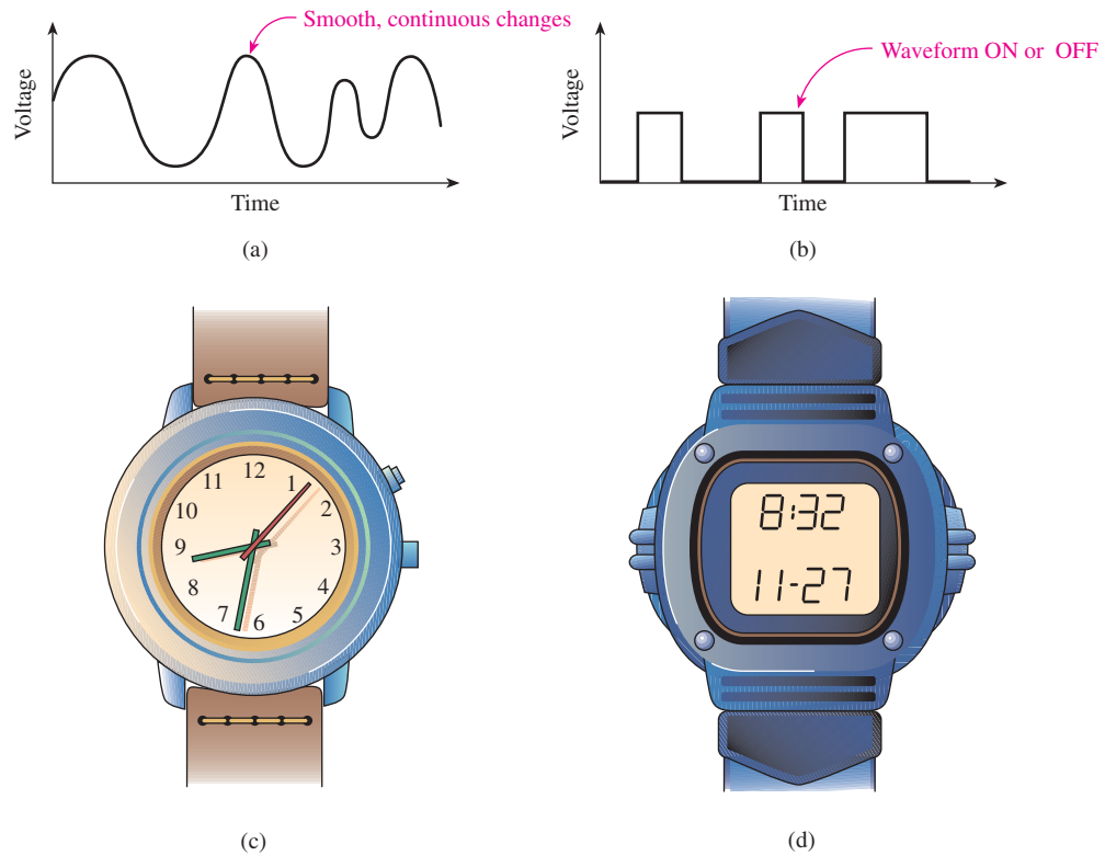
Figure 1 Analog versus digital: (a) analog waveform; (b) digital waveform; (c) analog watch; (d) digital watch.
