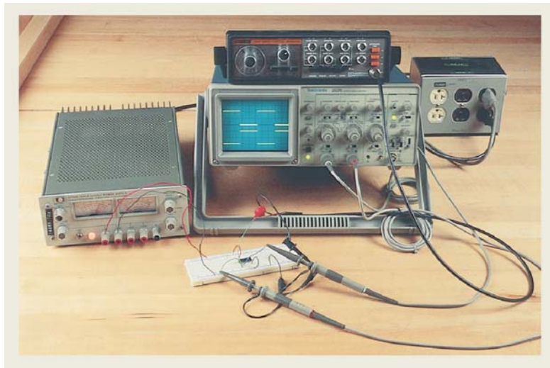
Figure 28 Timing analysis of an inverter gate: (a) waveform sketch and (b) oscilloscope display.
